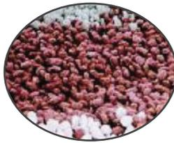
SEBS (Styrene Ethylene Butylene Styrene)
